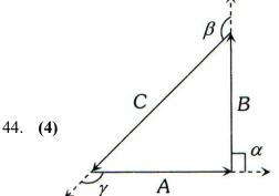
From polygon law, three vectors having summation zero should form a closed polygon (Triangle). Since the two vectors are having same magnitude and the third vector is  $\sqrt{2}$  times that of either of two having equal magnitude i.e. the triangle should be right angled triangle.
