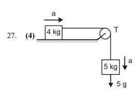
$$a = \frac{\text{Net driving force}}{\text{Total mass in motion}} = \frac{5g}{5+4} = \frac{5g}{9}$$
