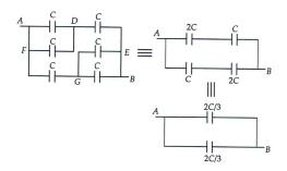
The equivalent capacitance between A and B is
